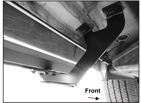
(Figure 9) Running Board attached to the driver/left front Mounting Bracket.
