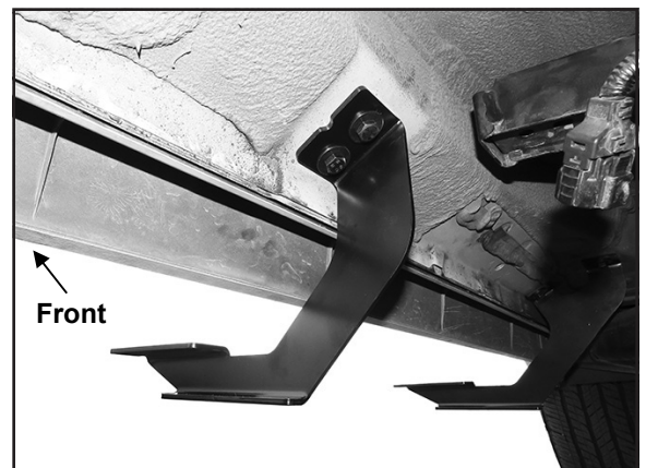
(Figure 4) Driver/left #2, #3 and Rear Bracket attached to the #2 location.
