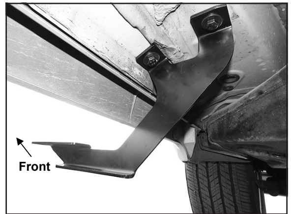
(Figure 3) Driver/left Front Mounting Bracket attached to the front location.
